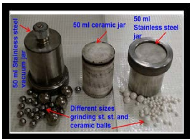
Figure 2: Ball mill accessories: Stainless steel vacuum jar, ceramic & stainless steel jar, stainless steel & ceramic grinding balls.
